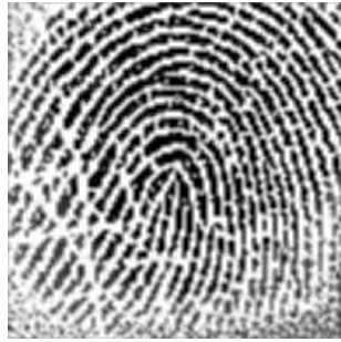
Figure 6. Example of a flat background fingerprint obtained from a thermoscanner.
